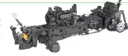
Optional factory installed front PTO, 3-point, and hydraulic valves make this the most multi-purpose tractor available
