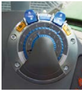
Intuitive operation with a compact power lift control module (EPC) and PTO control.
