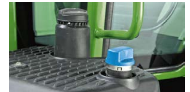
The 500 Vario has a 298 l capacity diesel tank which can work extensively without stopping. The AdBlue Tank is fully integrated into the diesel tank and holds 31 litres. Both tanks can be filled from the same side.
