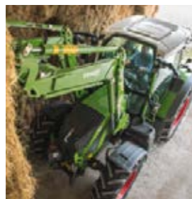
The panoramic windscreen with a full 77° field of vision upwards and over the wheel arches.
