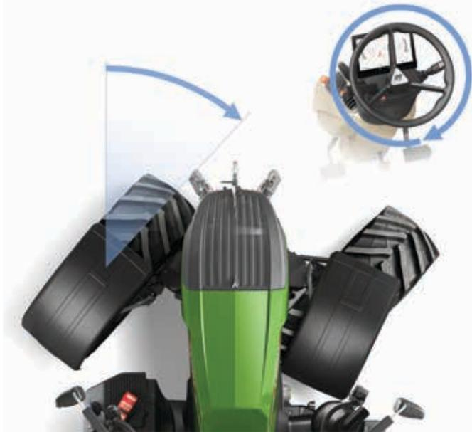
**Varioactive steering** reduces operator input and fatigue by requiring only a proportional turn of the steering wheel to achieve maximum steering angles. Steering sensitivity can easily be set and adjusted from the FendtONE displays.
