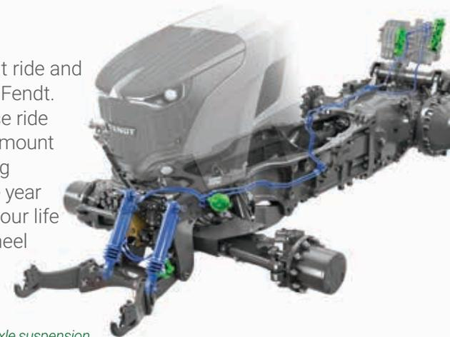
You'll never come up short with the Fendt hydraulic system. With up to 58 gallons per minute of dedicated hydraulic capacity, the Fendt 700 gives you the adaptability to work in multiple applications, no matter the demand.
