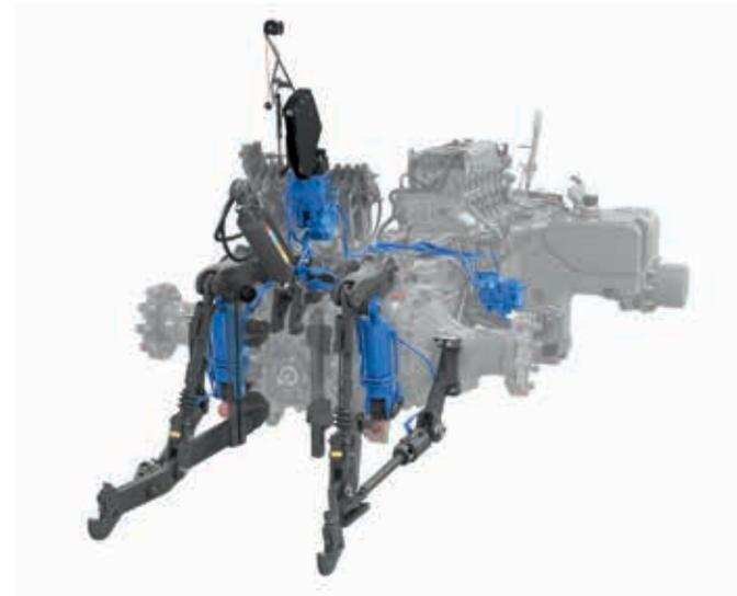
The rear 3-point features 24,000 lbs. of lift capacity and vibration dampening for smooth, easy transport.
