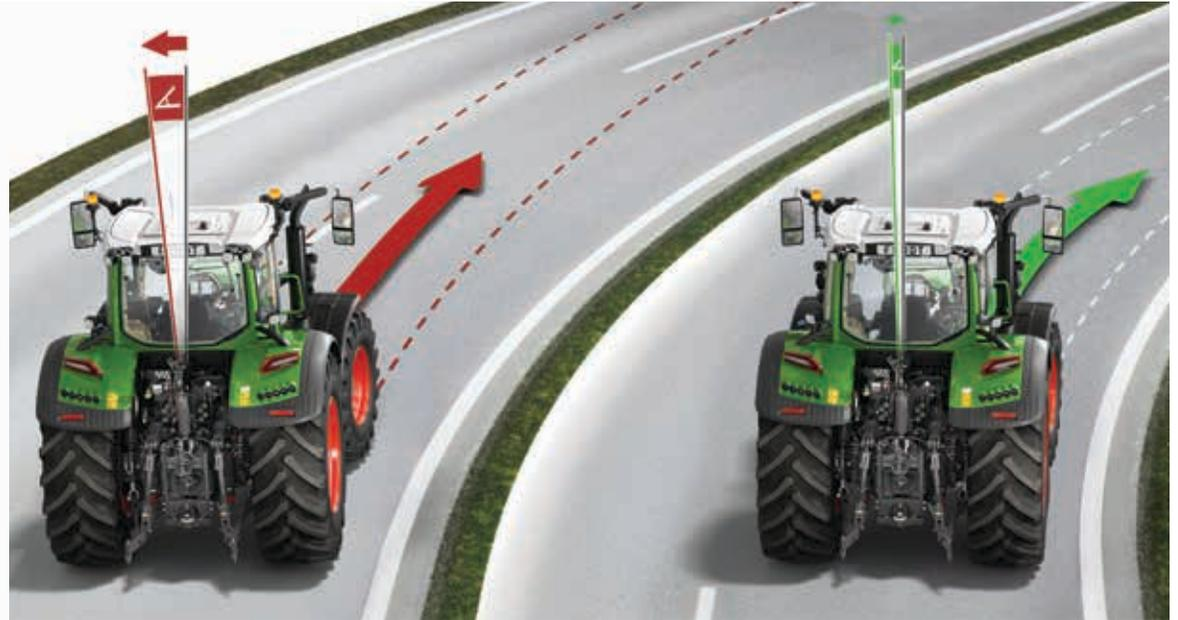
**Fendt Stability Control (FSC)** takes steering precision, driving stability and braking control to new levels. At speeds above 12.4 mph (20 km/h), FSC locks the front axle suspension cylinders and dampens side-to-side movement to ensure maximum stability in transport. When speeds drop below the FSC threshold, it automatically disengages to ensure maximum ground contact with all four tires.
