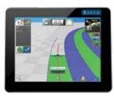
**CAMERA INTEGRATION** The Viper 4+ offers up to 4 camera connections. Monitor bin levels, blind spots, roadway operation and more right from your terminal.
